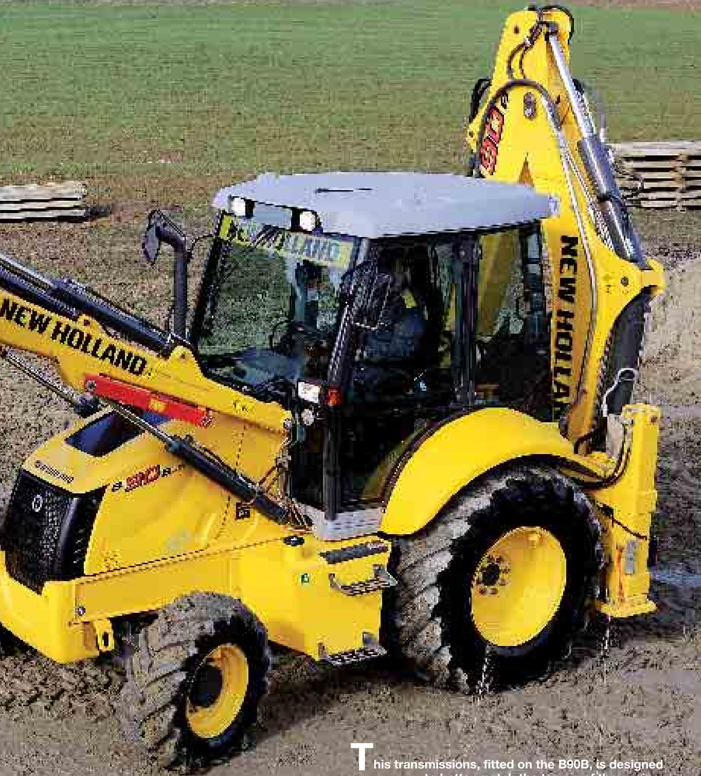
**T**his transmissions, fitted on the B90B, is designed to better match the torque of the engine. It efficiently follows the quicker response of the new engine to the operator demand and translates it into higher traction. This means shorter cycles and superior pushing capability in front loader operations, thus providing higher productivity and customer profit.
